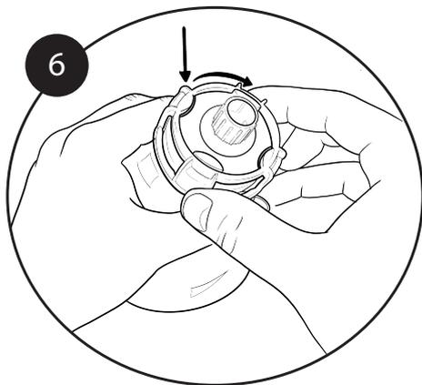
**6** Take the blue sealing ring and fit it to the pink bung. Align the tabs and push the ring onto the pink bung and twist to lock it in place.
